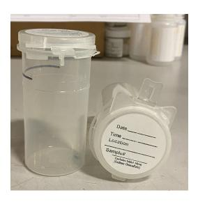
Coliform bottle 10mg tablet of Sodium Thiosulfate Aqueous samples
