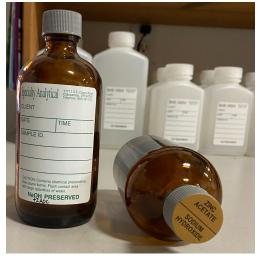
**125mL NaOH (Sodium Hydroxide) Preserved amber poly** Aqueous samples
